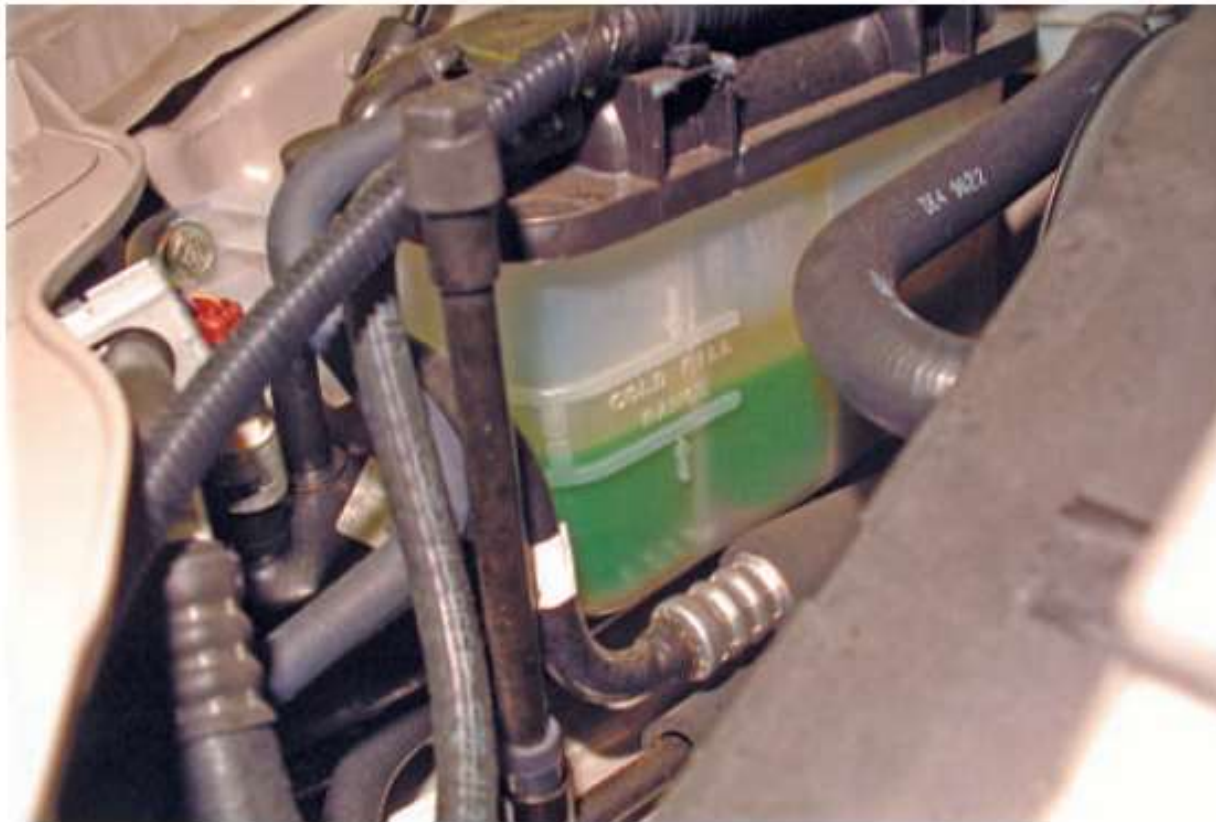
Figure 8-14 The level of coolant in the cooling system should be checked at the coolant recovery tank.
