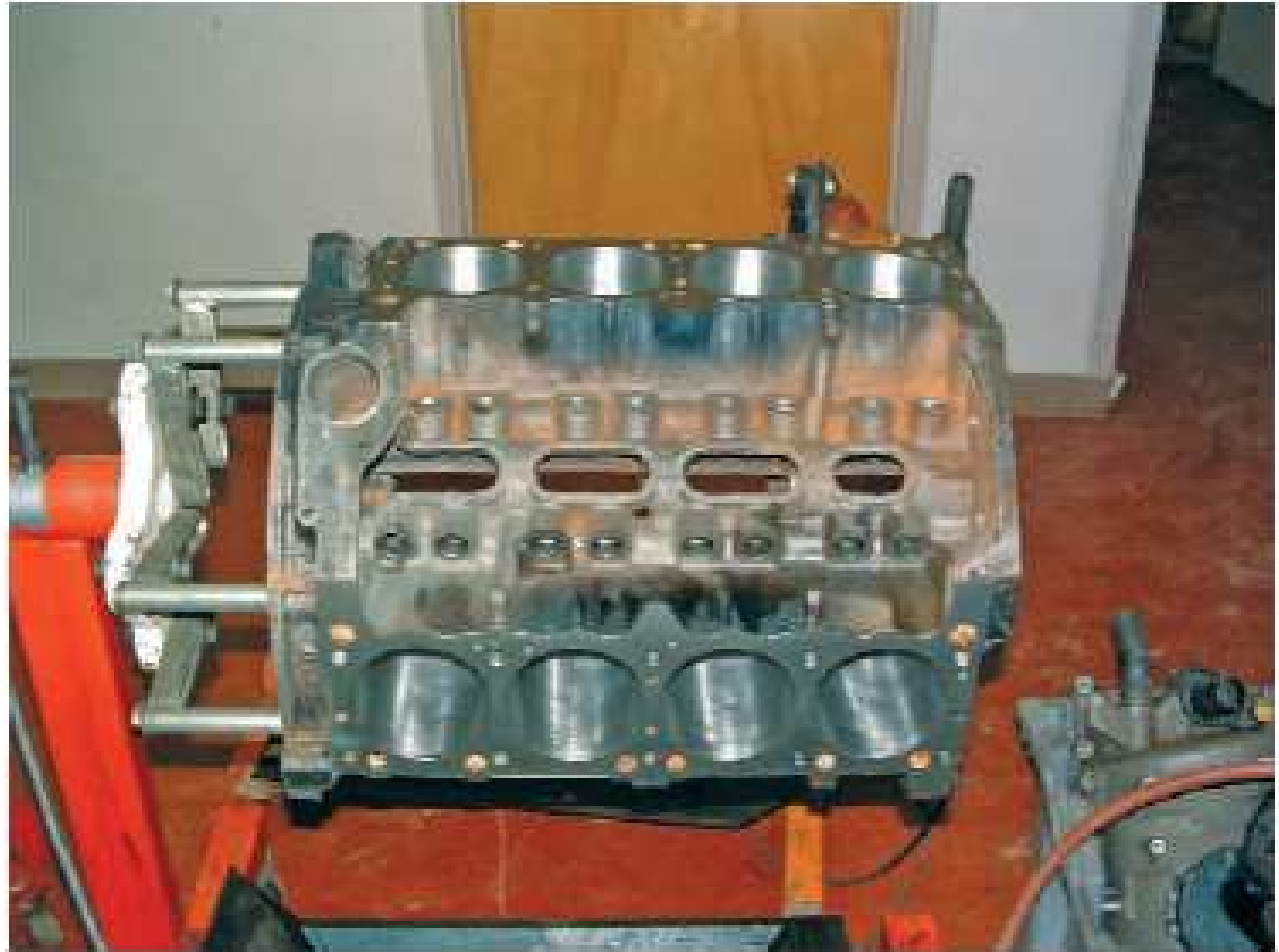
Figure 9-2 A cylinder block for an eight-cylinder engine.
