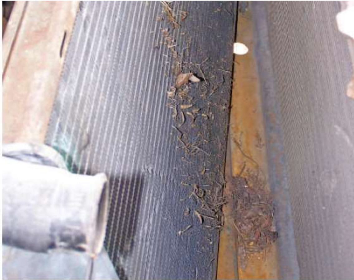
Figure 8-13 A buildup of dirt and bugs can restrict airflow through the radiator.
