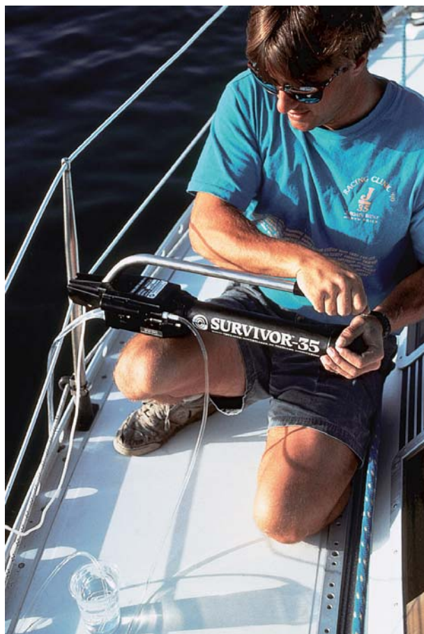
A small reverse-osmosis apparatus enables a person to obtain drinkable freshwater from seawater.
