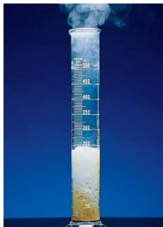
Figure 13.21 The decomposition of hydrogen peroxide is catalyzed by the iodide ion. A few drops of liquid soap have been added to the solution to dramatize the evolution of oxygen gas. (Some of the iodide ions are oxidized to molecular iodine, which then reacts with iodide ions to form the brown triiodide I_3^- ion.)
