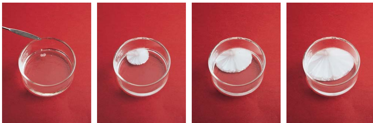
Figure 12.1 In a supersaturated sodium acetate solution (left), sodium acetate crystals rapidly form when a small seed crystal is added.
