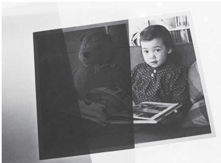
Figure 22.15 With one Polaroid sheet over a picture, light passes through. With a second sheet of Polaroid placed over the first so that the axes of polarization of the sheets are perpendicular, little or no light passes through. If the axes of polarization of the two sheets were parallel, light would pass through.
