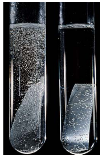
Zn reacts more vigorously with a strong acid like HCl (left) than with a weak acid like CH 3 COOH (right) of the same concentration because there are more H + ions in the former solution.
