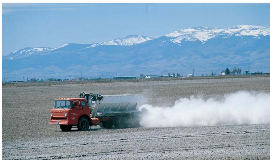
Figure 17.24 Spreading calcium oxide ( \text{CaO} ) over acidified soil. This process is called liming.
