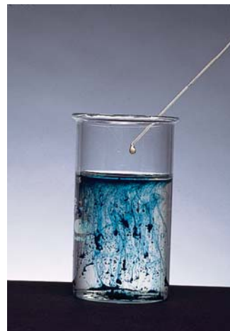
Prussian blue can be prepared by mixing a \text{FeCl}_3 solution with a \text{K}_4\text{Fe}(\text{CN})_6 solution.
