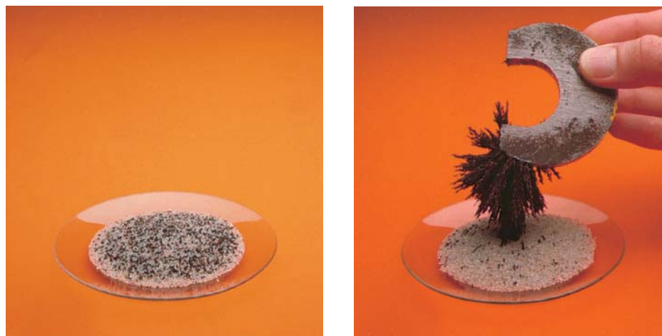
Figure 1.4 (a) The mixture contains iron filings and sand. (b) A magnet separates the iron filings from the mixture. The same technique is used on a larger scale to separate iron and steel from nonmagnetic objects such as aluminum, glass, and plastics.
