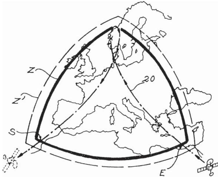
Figure 2.19 Zone of coverage with an elevation angle greater than 55^\circ (two satellites in Tundra orbits). Source: after [ROU-88]. Reproduced by permission of the Institution of Electrical Engineers.
