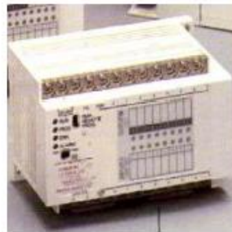
Micro PLC - handles up to 32 I/O points
