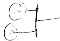
$$\frac{2H_1}{w_s} \frac{d^2\delta_1}{dt^2} = P_{m1} - P_{e1} \text{ pu}$$
