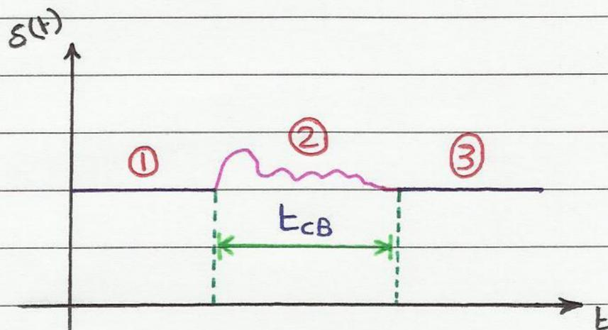
$t_{CB}$  is time for circuit breaker to disconnect.
