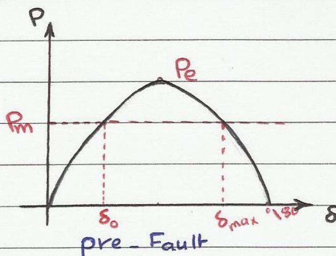
\* When the Fault occurs, the electrical power output is suddenly zero while the input mechanical power is unaltered.
