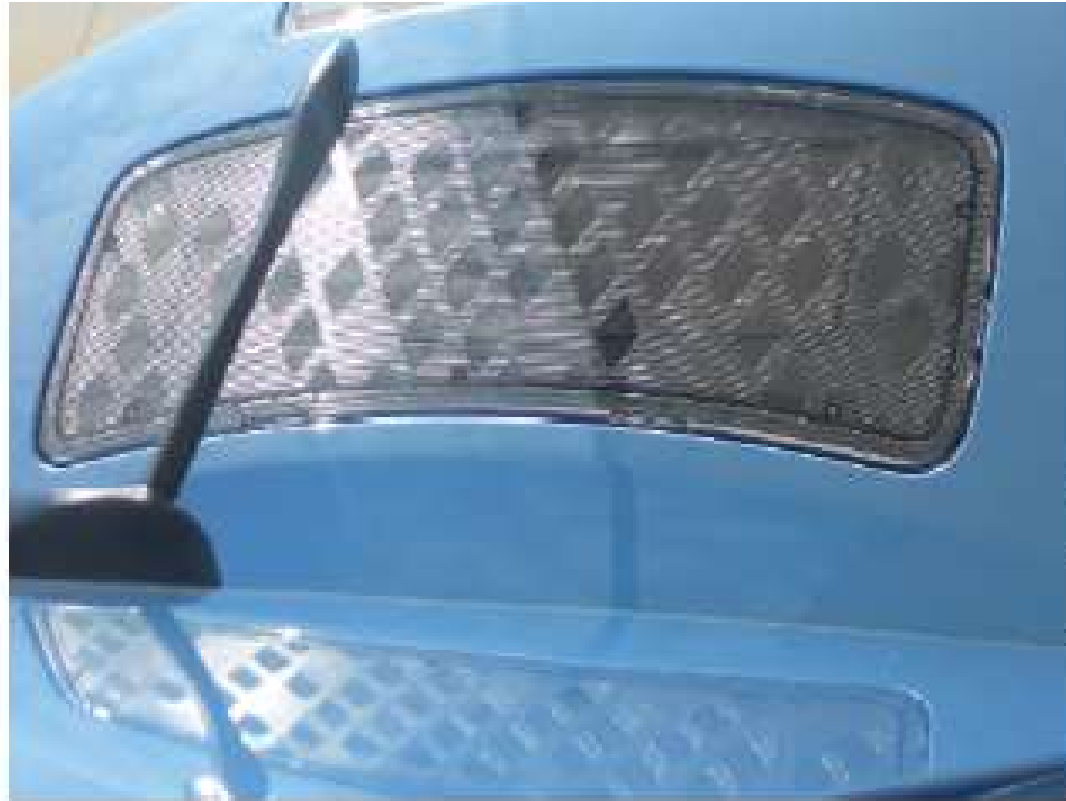
Figure 36-25 The solar panel built into the spoiler on some models of the Leaf.
