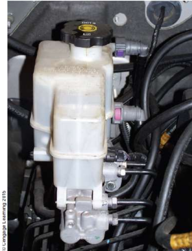
Figure 36-16 The master cylinder and pump assembly for an electro-hydraulic brake system.
