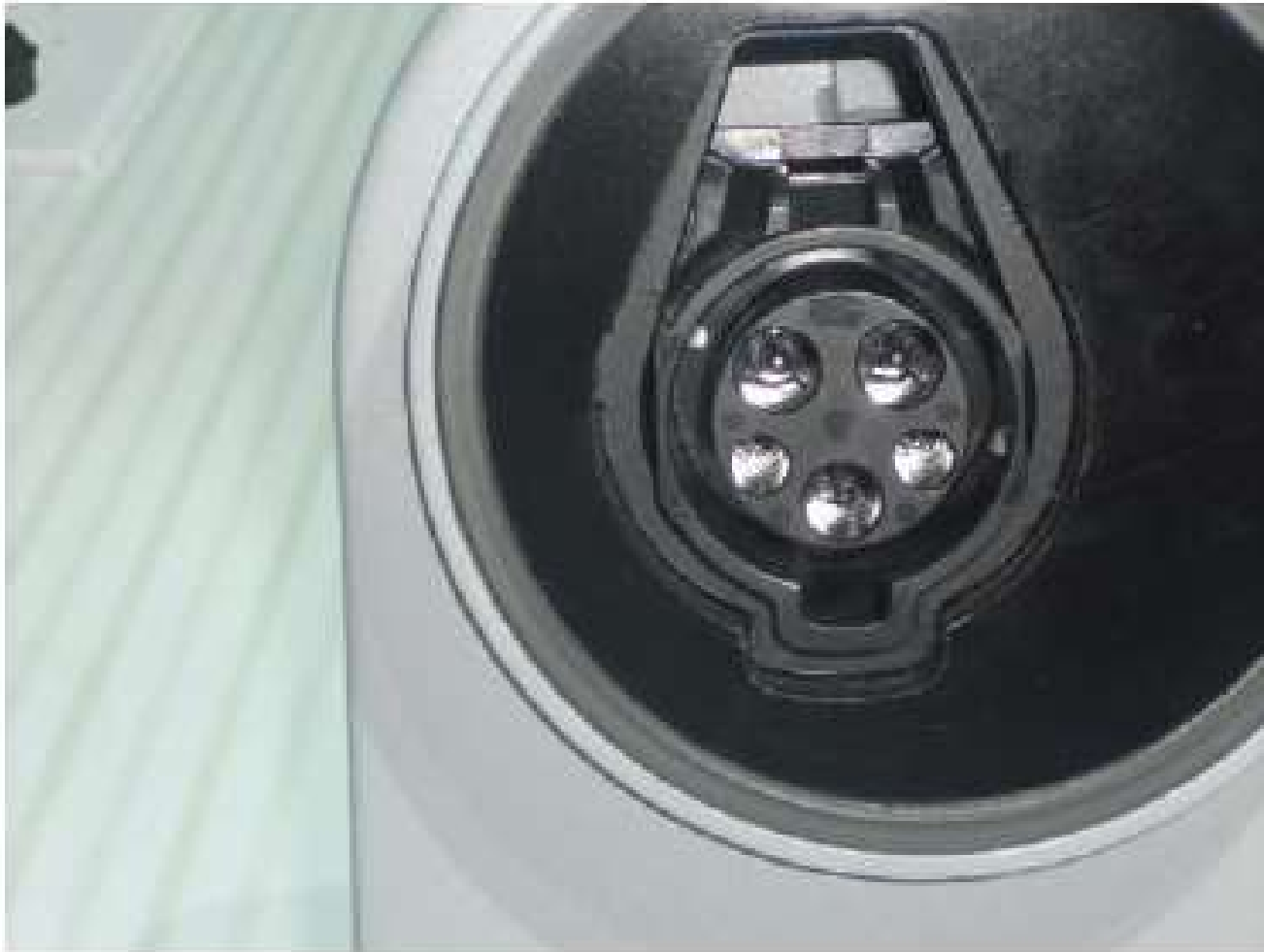
Figure 36-13 The female connections for a SAE J1772 connector.
