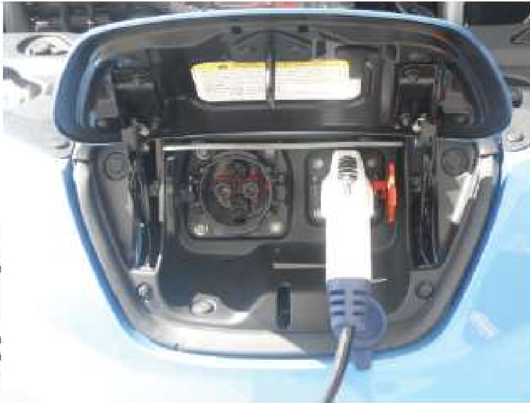
Figure 36-24 The Leaf's charging port at the front of the car and the two charging inlets.
