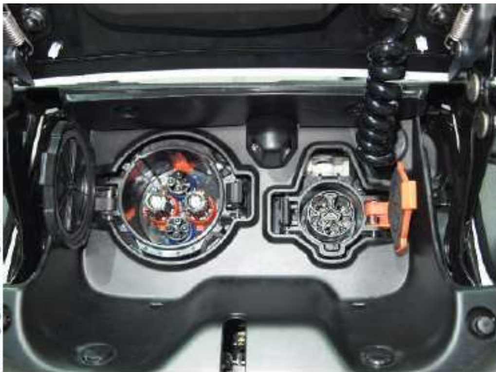
Figure 36-15 The Nissan Leaf has receptacles for a CHAdeMO and SAE J1772 connector.
