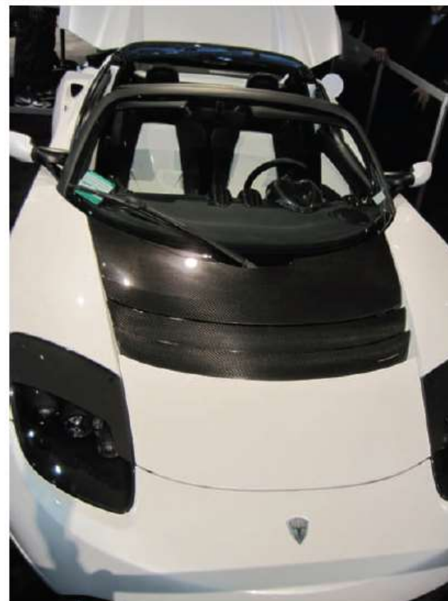
Figure 36-28 The Tesla Roadster is an EV based on the gasoline-powered Lotus Elise.
