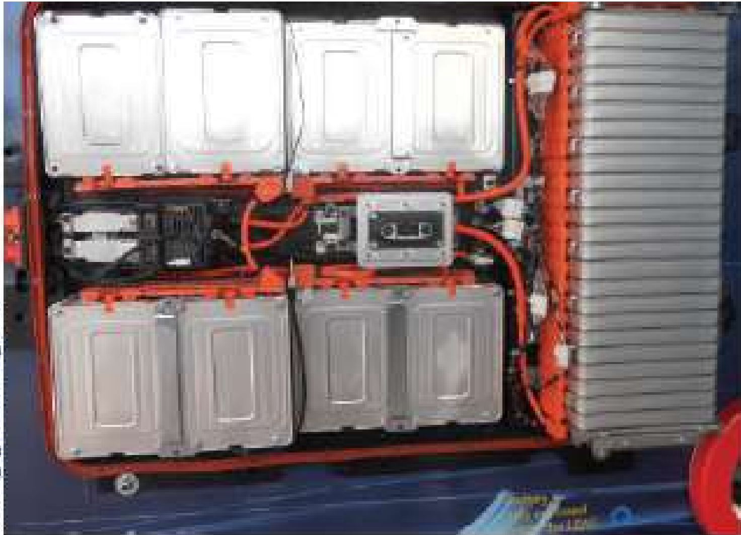
Figure 36-23 The battery pack in a Leaf.
