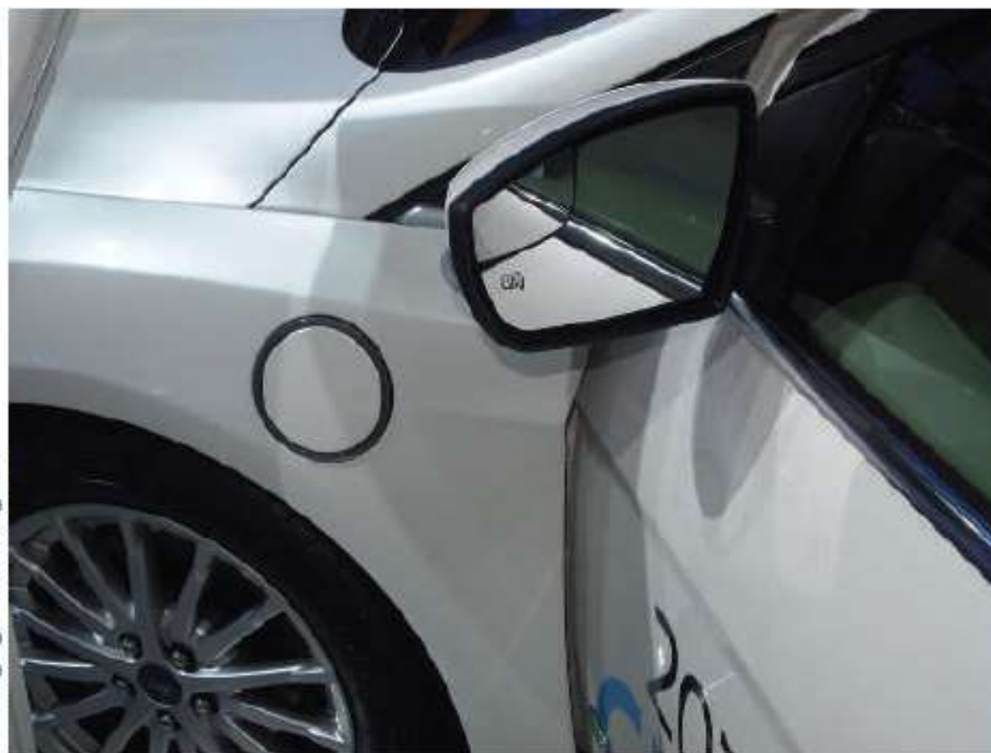
Figure 36-21 The charging port on a Focus is on the left front fender.
