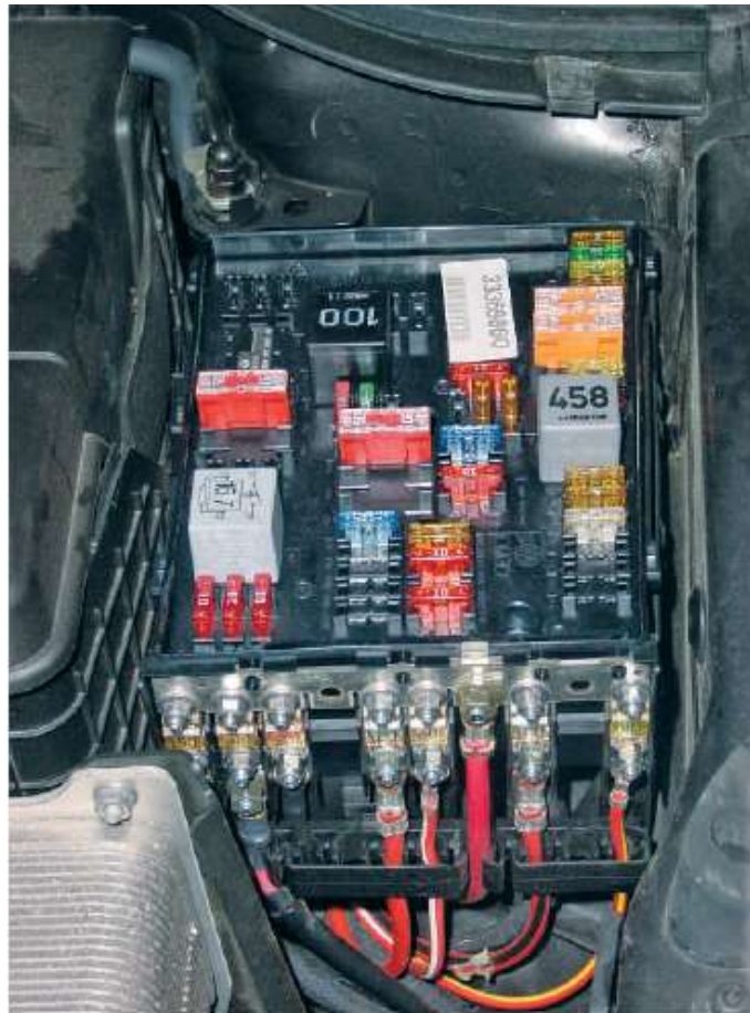
Figure 15-43 Typical fuse box or panel.
