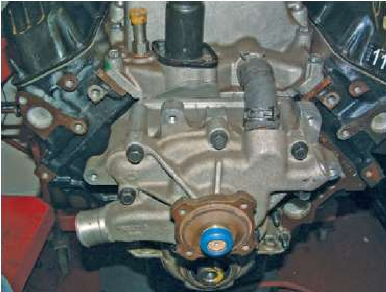
Figure 14-26 A water pump bolted to the front of an engine.
