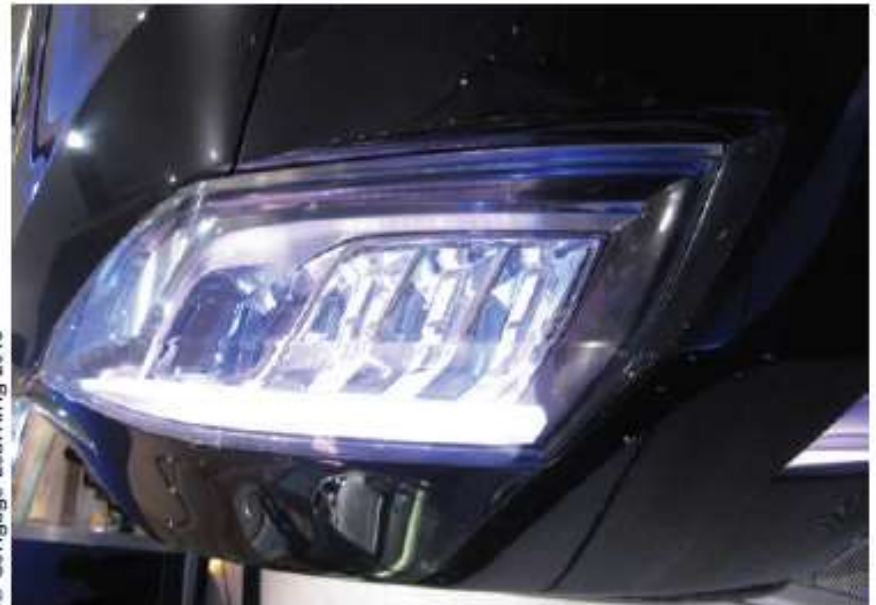
Figure 20-12 HID (xenon) headlights are readily identifiable by their bluish light.
