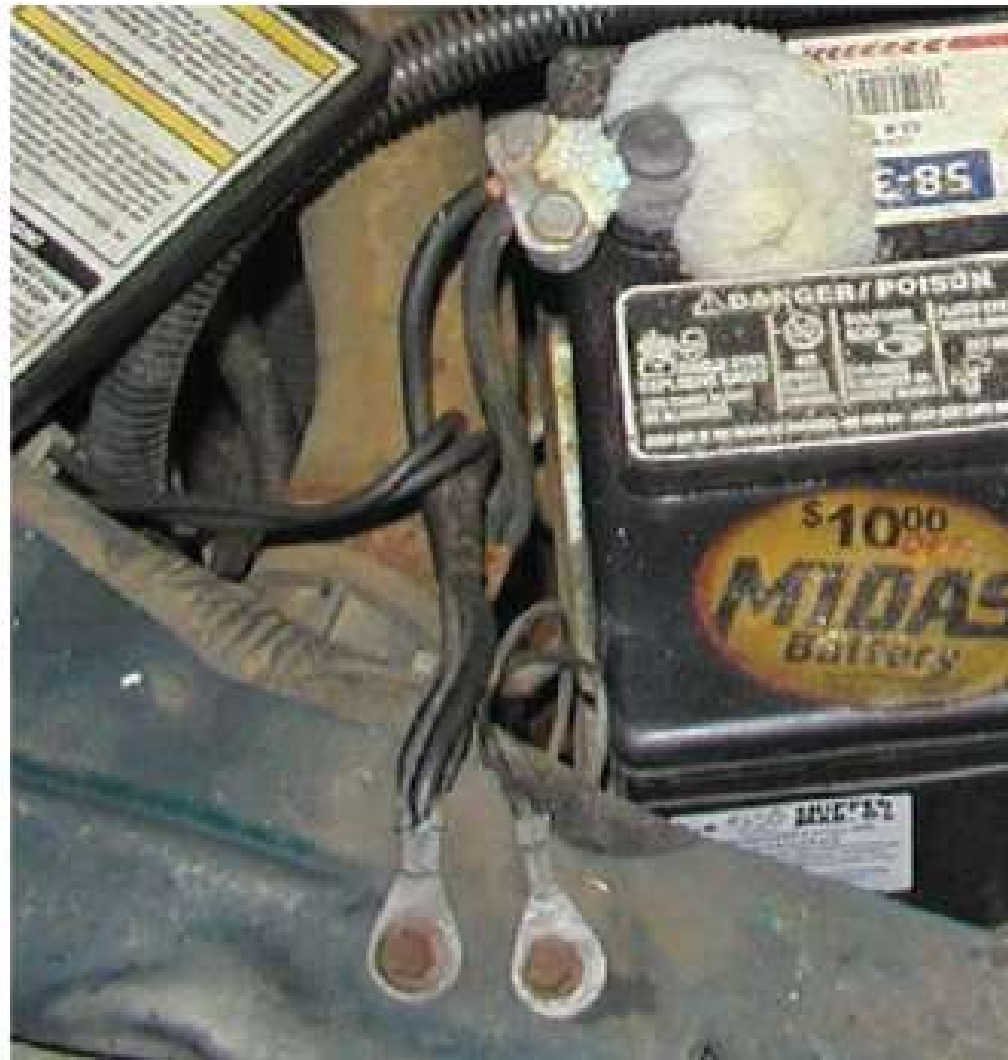
Figure 15-15 Chassis ground connections for a very dirty battery.
