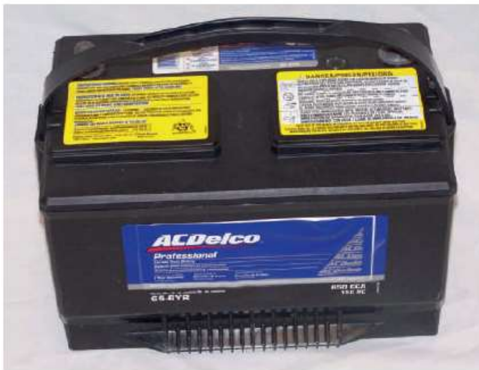
Figure 17-1 A typical 12-volt battery.
