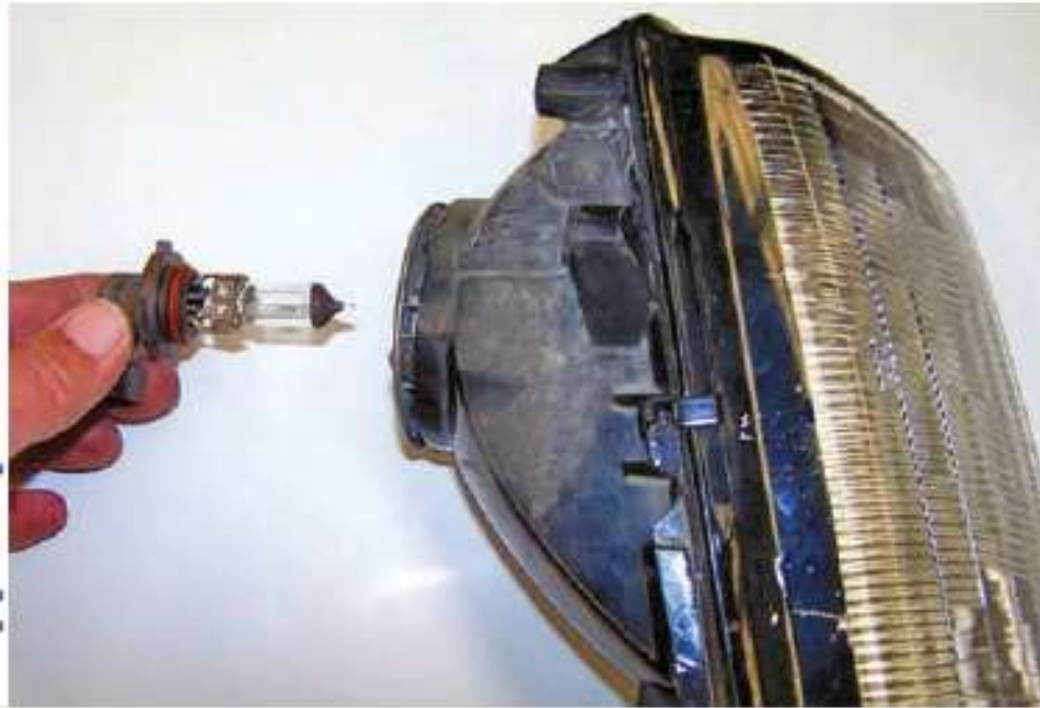
Figure 20-10 A composite headlamp with a replaceable halogen bulb.
