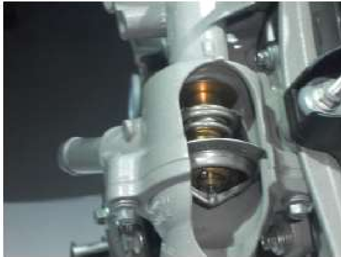
Figure 14-25 A typical thermostat located in the water outlet.
