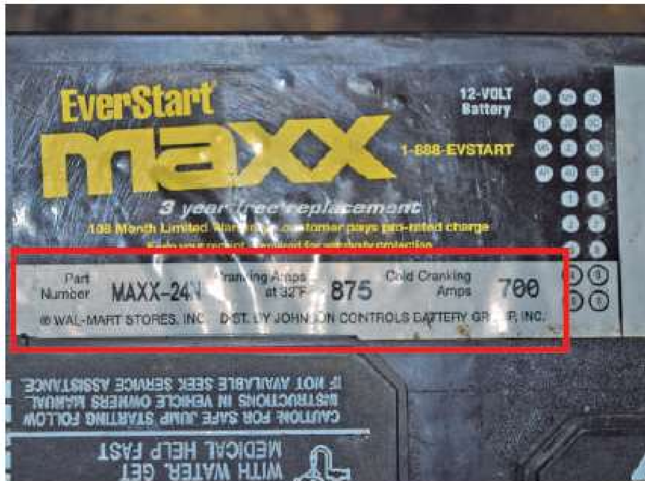
Figure 17-10 The sticker on this battery shows its CA and CCA ratings.
