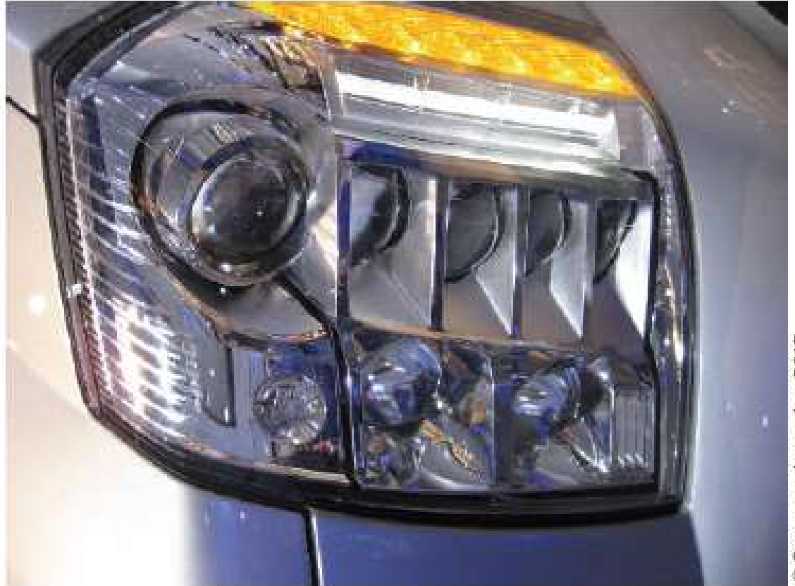
Figure 20-19 A headlight assembly of HID bulbs and LEDs.
