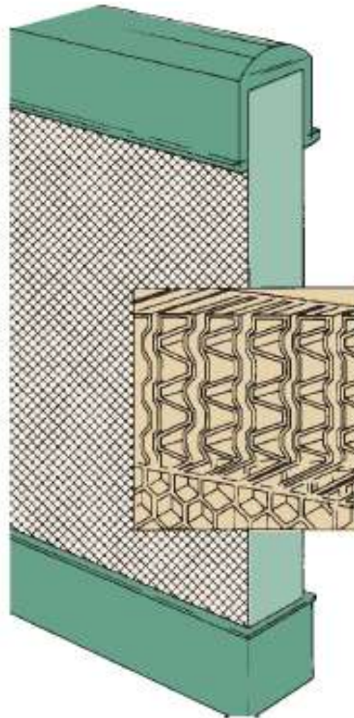
Figure 14-29 A radiator core is made of a series of tubes and fins that expose the coolant's heat to as much surface area as possible.
