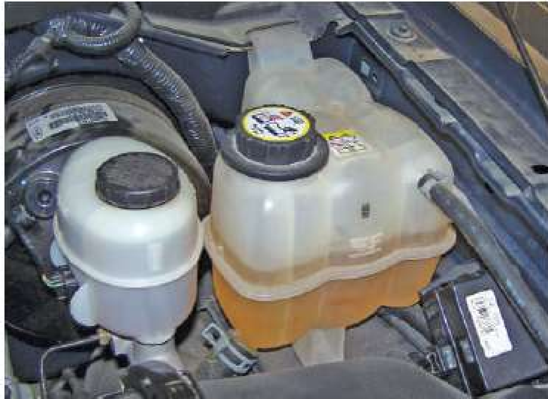
Figure 14-33 A coolant expansion tank.
