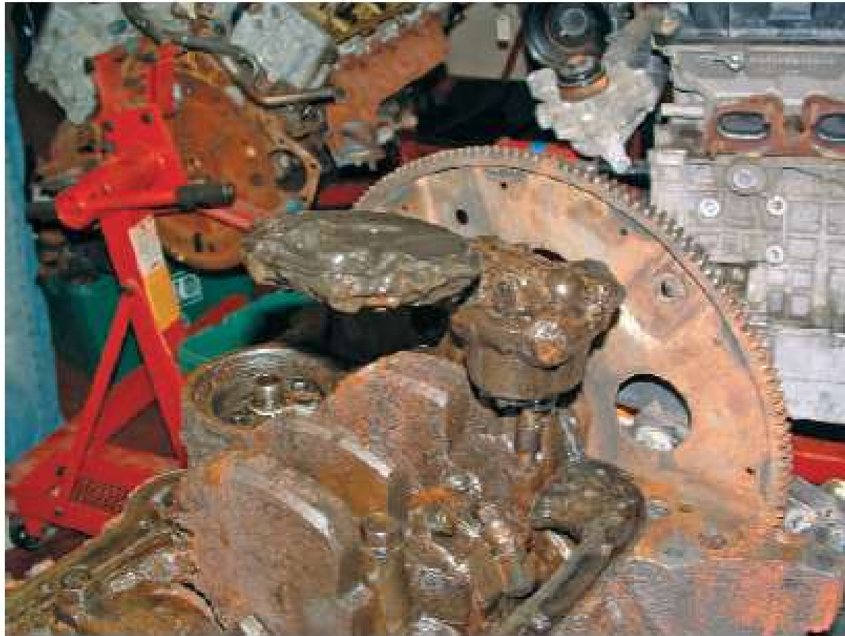
Figure 14-22 Sludge buildup on the lower parts of an engine.
