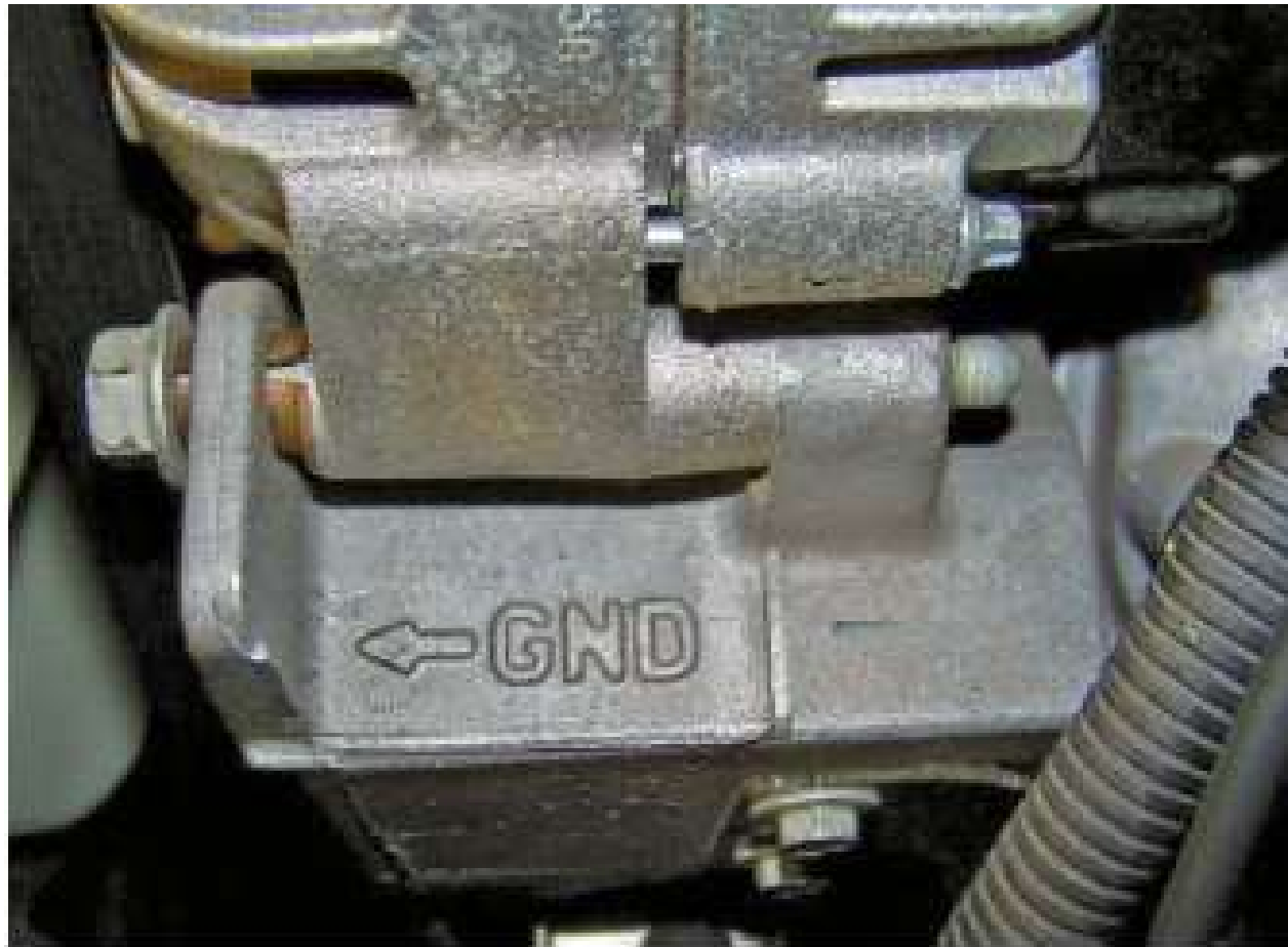
Figure 15-14 Many electrical parts are grounded through their mounting to the engine, transmission, or frame.
