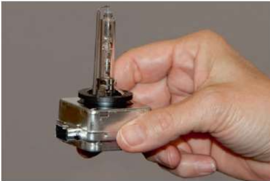
Figure 20-11 A xenon light bulb.
