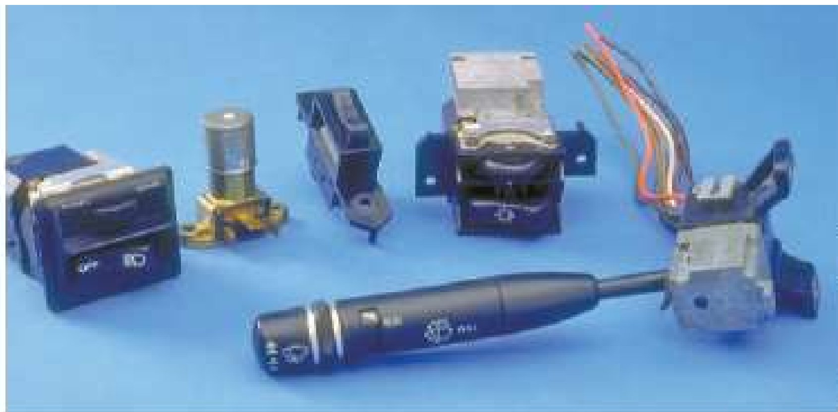
Figure 15-48 Examples of the various switches used in automobiles.
