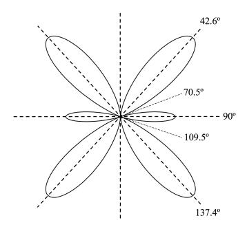
b) Determine the sidelobe level, as per the definition in Problem 14.15: At the main lobe angle  $(\theta = 42.6^{\circ})$ ,  $[F(\theta)]^2$  evaluates as 1.96. The sidelobe at  $\theta = 90^{\circ}$  gives a value of 1.00. The sidelobe level in decibles is thus
