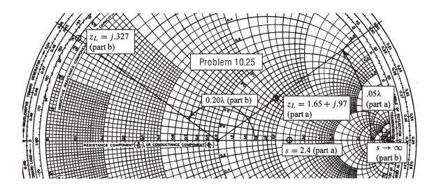
10.26. A 50-ohm lossless line is of length  $1.1\lambda$ . It is terminated by an unknown load impedance. The input end of the 50-ohm line is attached to the load end of a lossless 75-ohm line. A VSWR of 4 is measured on the 75-ohm line, on which the first voltage maximum occurs at a distance of  $0.2\lambda$  in front of the junction between the two lines. Use the Smith chart to find the unknown load impedance.
