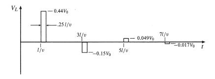
10.40. In the charged line of Fig. 10.25, the characteristic impedance is  $Z_0 = 100\Omega$ , and  $R_g = 300\Omega$ . The line is charged to initial voltage  $V_0 = 160$  V, and the switch is closed at t = 0. Determine and plot the voltage and current through the resistor for time 0 < t < 8l/v (four round trips). This problem accompanies Example 11.12 as the other special case of the basic charged line problem, in which now  $R_g > Z_0$ . On closing the switch, the initial voltage wave is
