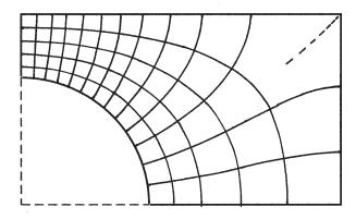
b) Assume  $\epsilon = \epsilon_0$  and estimate C per meter length: In this case  $N_Q$  is the number of squares around the full perimeter of the circular conductor, or four times the number of squares shown in the drawing.  $N_V$  is the number of squares between the circle and the rectangle, or 5. The capacitance is estimated to be
