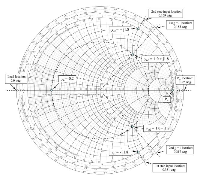
**10.33.** In Fig. 10.17, let  $Z_L = 40 - j10 \Omega$ ,  $Z_0 = 50 \Omega$ , f = 800 MHz, and v = c.
