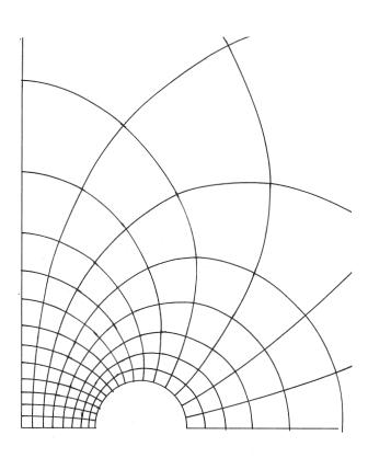
**6.19.** Construct a curvilinear square map of the potential field between two parallel circular cylinders, one of 4-cm radius inside one of 8-cm radius. The two axes are displaced by 2.5 cm. These dimensions are suitable for the drawing. As a check on the accuracy, compute the capacitance per meter from the sketch and from the exact expression:
