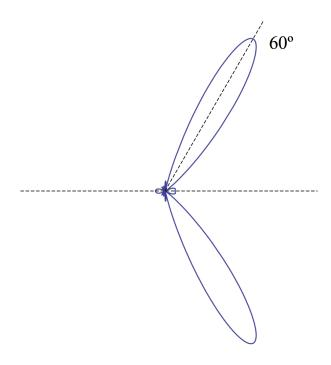
**14.26.** In a linear endfire array of n elements, a choice of current phasing that improves the directivity is given by the Hansen-Woodyard condition:
