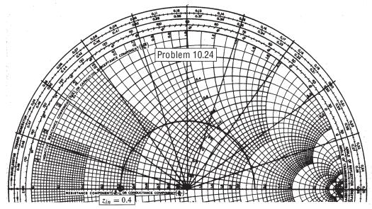
On the chart, radial lines are drawn at positions corresponding to  $.025\lambda$  increments on the WTG scale. The intersections of the lines and the circle give a total of 11  $z_{in}$  values. To these we add normalized impedance of 40/50 = 0.8 to add the effect of the  $40\Omega$  resistors and obtain the normalized impedance at the line input. The magnitudes of these values are then found, and the results are multiplied by  $50\Omega$ . The table below summarizes the results.
