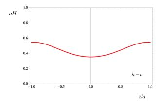
Which choice for h gives the most uniform field? From the results, h = a/2 is evidently the best. This is the Helmholtz coil configuration – in which the spacing is equal to the coil radius.
