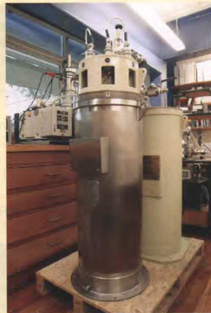
■ FIGURE 13.29 Prototype 15 kVA partial core superconducting power transformer.
