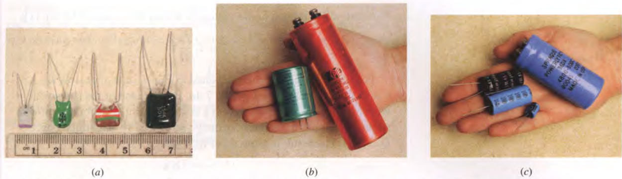
FIGURE 7.2 Several examples of commercially available capacitors. (a) Left to right: 270 pF ceramic, 20 \mu\text{F} tantalum, 15 nF polyester, 150 nF polyester. (b) Left: 2000 \mu\text{F} 40 VDC rated electrolytic, 25,000 \mu\text{F} 35 VDC rated electrolytic. (c) Clockwise from smallest: 100 \mu\text{F} 63 VDC rated electrolytic, 2200 \mu\text{F} 50 VDC rated electrolytic, 55 F 2.5 VDC rated electrolytic, and 4800 \mu\text{F} 50 VDC rated electrolytic. Note that generally speaking larger capacitance values require larger packages, with one notable exception above. What was the tradeoff in that case?
