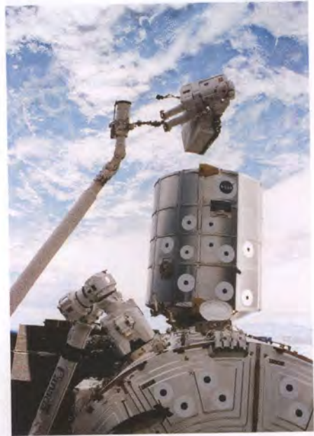
An example of a robotic manipulator. The feedback control system can be modeled using linear circuit elements to determine situations in which the operation may become unstable. (NASA Marshall Space Flight Center.)
