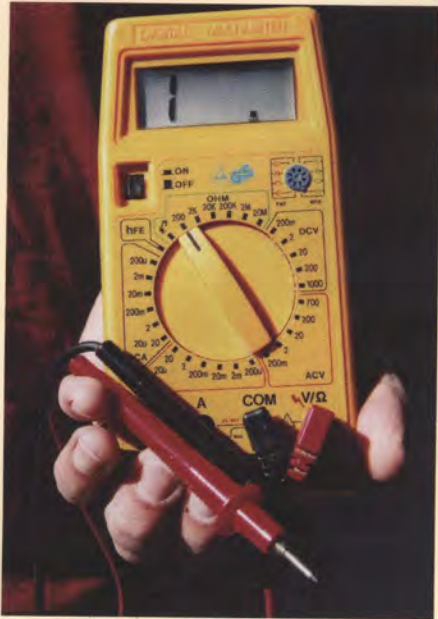
■ FIGURE 5.34 A handheld digital multimeter.
