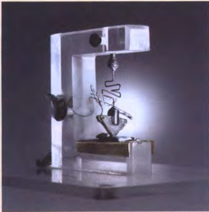
■ FIGURE 17.24 Photograph of the first demonstrated bipolar junction transistor (“bjt”). Lucent Technologies Inc./Bell Labs
