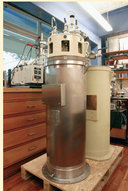
■ FIGURE 13.29 Prototype 15 kVA partial core superconducting power transformer. (Courtesy of Department of Electrical and Computer Engineering, University of Canterbury)
