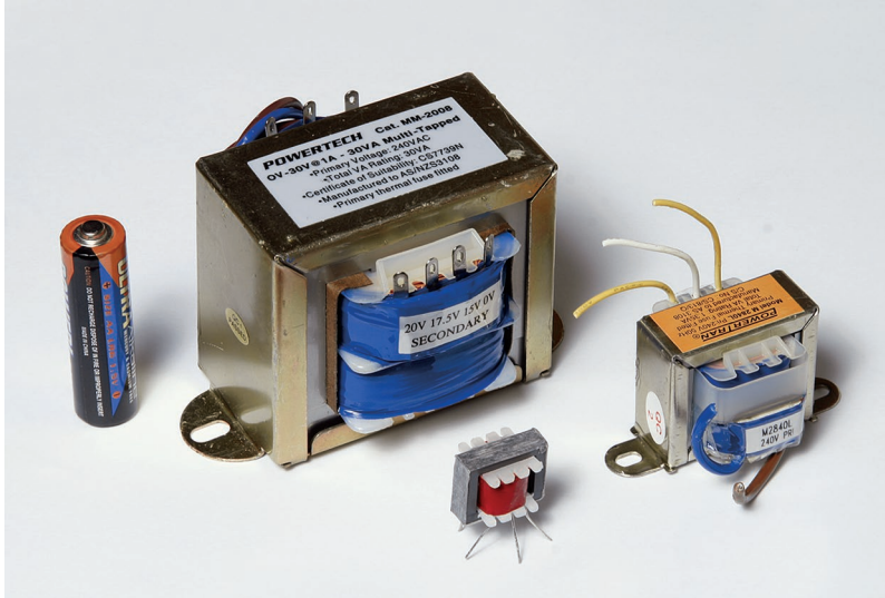
■ FIGURE 13.15 A selection of small transformers for use in electronic applications; the AA battery is shown for scale only. (©Steve Durbin)
