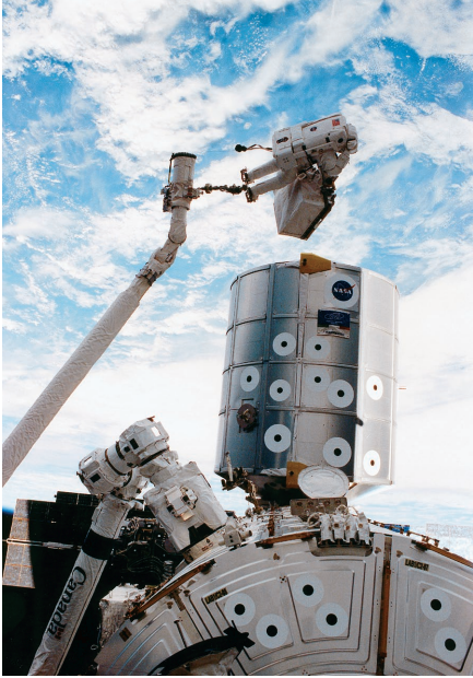
An example of a robotic manipulator. The feedback control system can be modeled using linear circuit elements to determine situations in which the operation may become unstable. (Source: NASA Marshall Space Flight Center)
