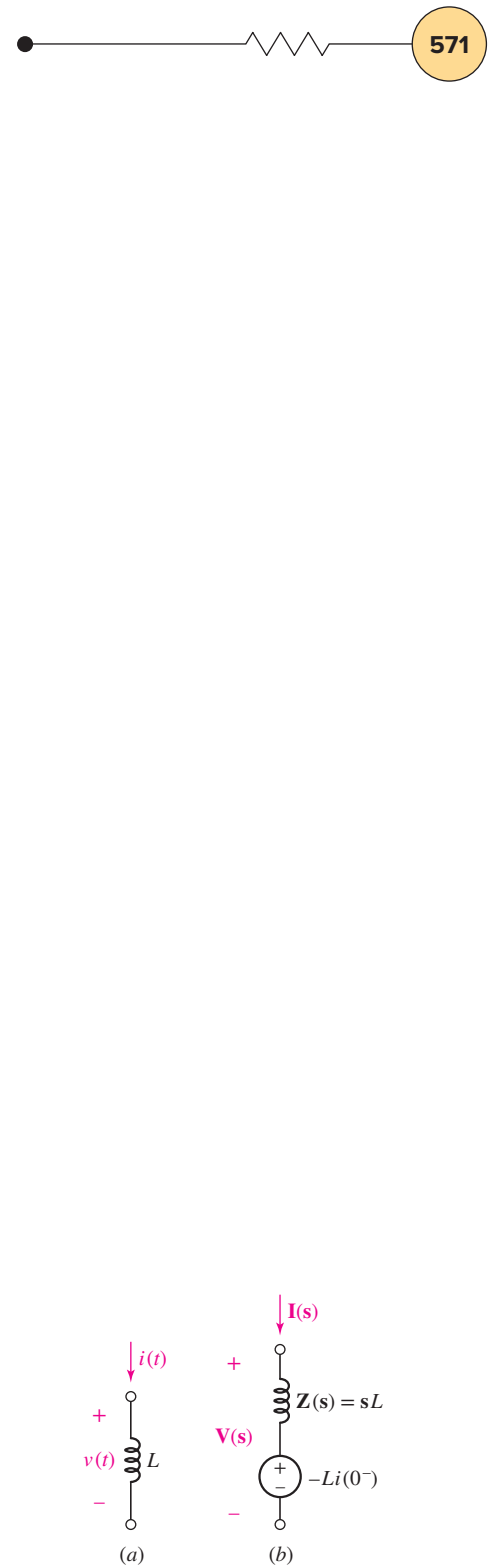
FIGURE 14.9 (a) Inductor in the time domain. (b) The complete model for an inductor in the frequency domain, consisting of an impedance sL and a voltage source -Li(0^-) that incorporates the effects of nonzero initial conditions on the element.
