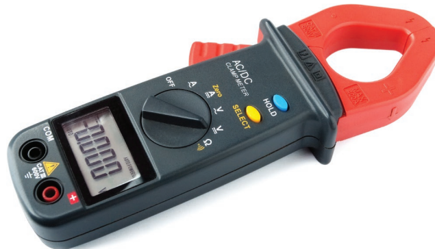
■ FIGURE 11.19 Example of a clamp-on digital power meter capable of measuring ac currents and voltages. (©KhotenkoVolodymyr/Getty Images)
