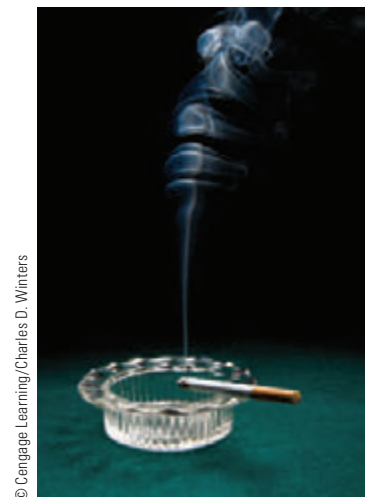
Figure 14.14 Hot gases from a cigarette made visible by smoke particles. The smoke first moves in laminar flow at the bottom and then in turbulent flow above.
