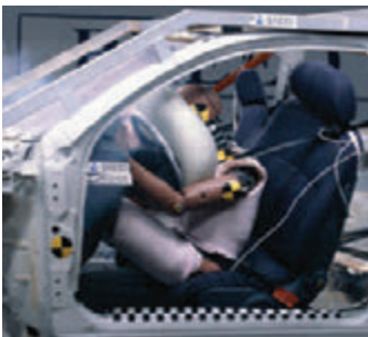
Air bags in automobiles have saved countless lives in accidents. The air bag increases the time interval during which the passenger is brought to rest, thereby decreasing the force on (and resultant injury to) the passenger.
