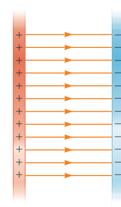
Figure 24.15 (Example 24.5) The electric field lines between two infinite planes of charge, one positive and one negative. In practice, the field lines near the edges of finite-sized sheets of charge will curve outward.
