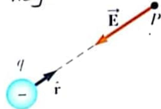
6) The force on a positive charge is in the same direction of  $\vec{E}$
