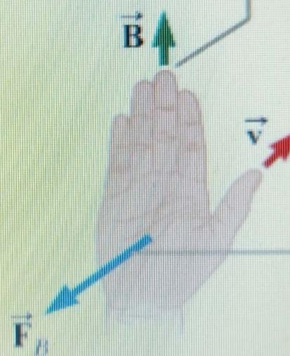
(2) The magnetic force on a positive particle is in the direction you would push with your palm.
