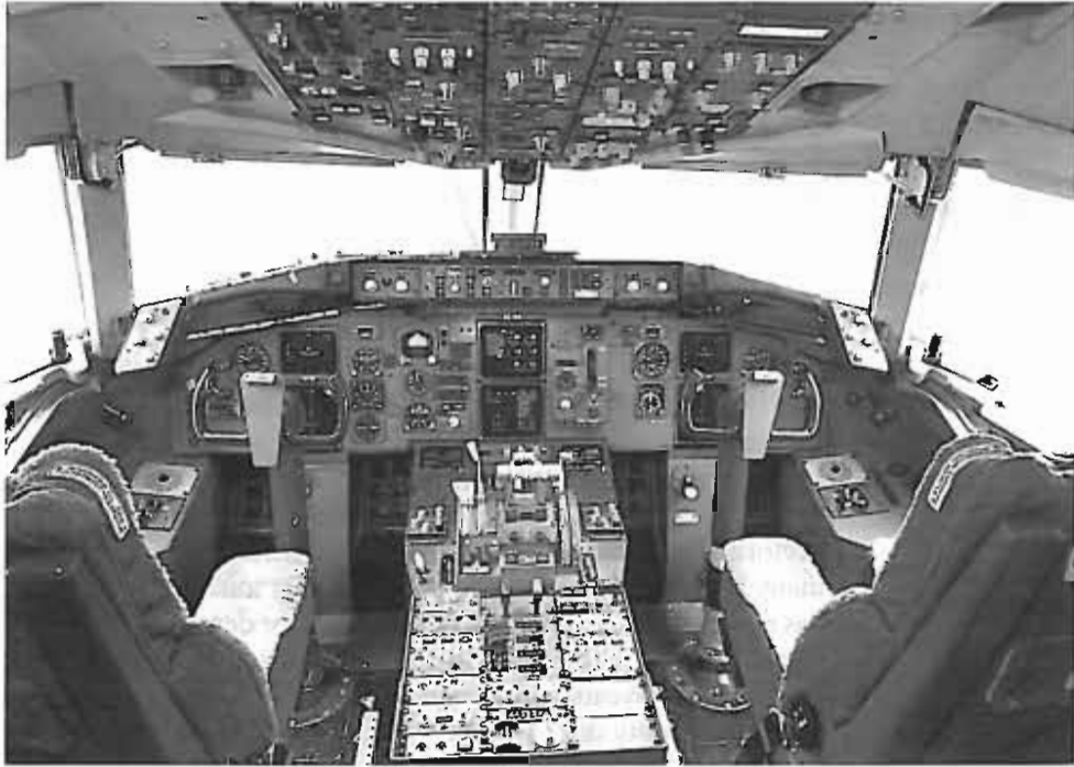
FIGURE 13.3 The flight deck of the Boeing 757 and 767 features digital control electronics, including an engine indicating system and a crew alerting system. All systems controls are within reach of either pilot. The system includes an inertial reference system making use of laser gyroscopes and an electronic attitude director indicator. A flight-management computer system integrates navigation, guidance, and performance data functions. When coupled with the automatic flight control system (automatic pilot), the flight-management system provides accurate engine thrust settings and flight-path guidance during all phases of flight from immediately after takeoff to final approach and landing. The system can predict the speeds and altitudes that will result in the best fuel economy and command the airplane to follow the most fuel-efficient or the “least time” flight paths. (Courtesy of Boeing Airplane Co.)
