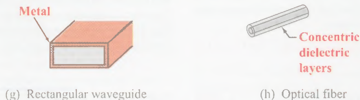
Figure 2-4: A few examples of transverse electromagnetic (TEM) and higher-order transmission lines.
