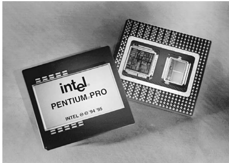
Figure 67 Pentium Pro processor IC. (Reprinted by permission of Intel Corporation. Copyright/ Intel Corp. 1996)
