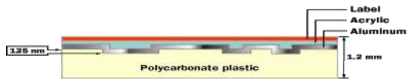
Figure 6.4: cross section of a CD
