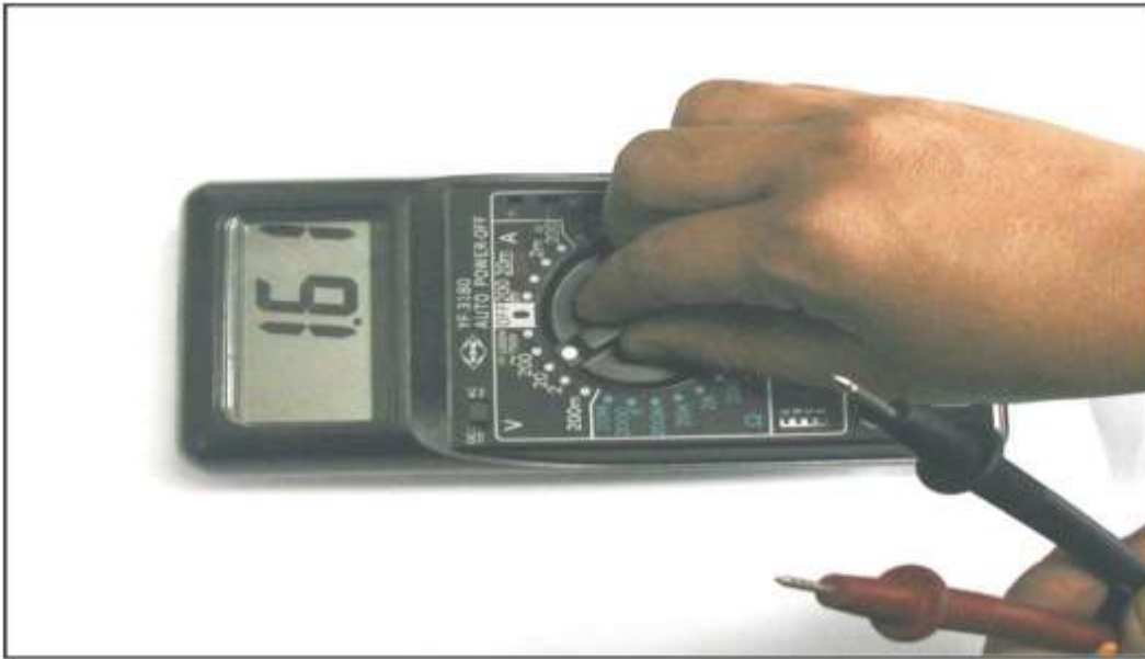
Figure 4.2 Voltage mode setting on multimeter.
