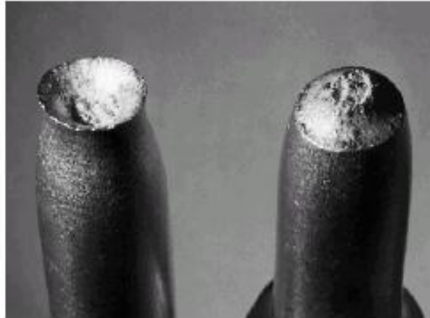
(Cap-and-cone fracture in Al)
