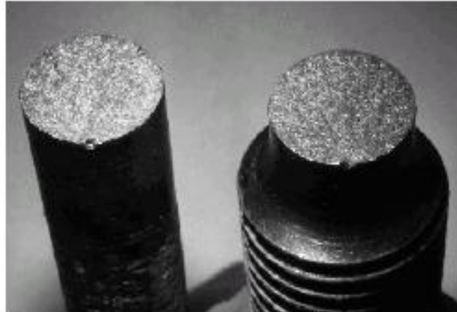
Brittle fracture in a mild steel
