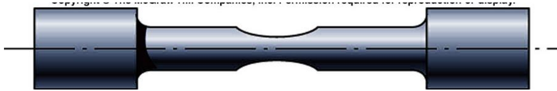
Necking of ductile material under tensile load
