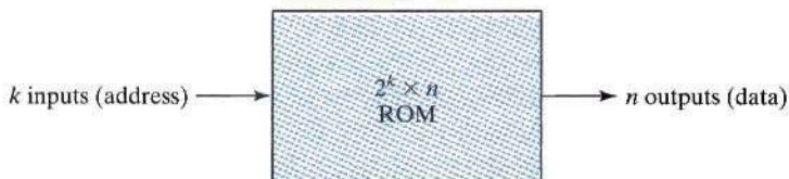
FIGURE 7.9 ROM block diagram
