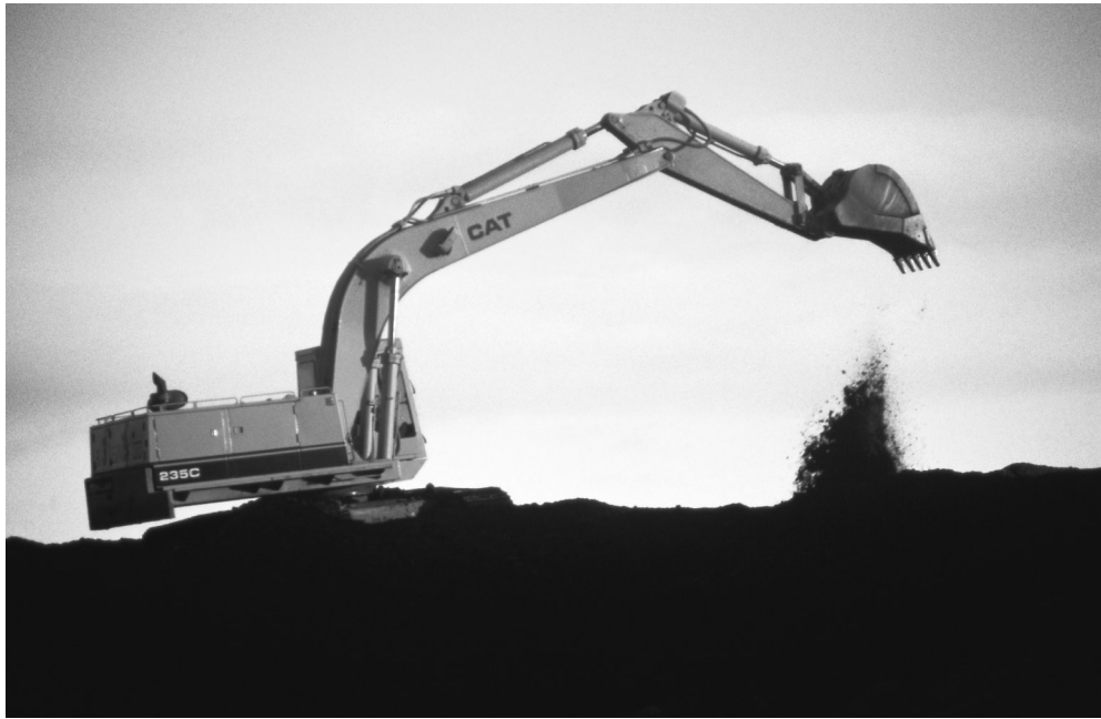
FIGURE 1.34 The motion of this backhoe is determined by several independently controlled mechanisms. (Source: Caterpillar.)
