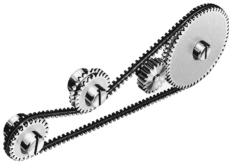
FIGURE 8.29 Positive-drive belt used with geared pulleys. The reinforced plastic belt was originally developed as a silent drive for sound and recording systems. The geared pulleys may be directly meshed with spur gears, eliminating intermediate components. An idler is usually used as shown to take up the slack. The flexibility of this type of belt allows for considerable shaft misalignment, and, with idlers or guides, the belt may even be used between pulleys on perpendicular intersecting shafts. (Source: Precision Industrial Components Corporation, Wells-Benrus Corporation.)
