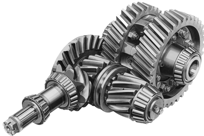
FIGURE 7.2 A speed reducer employing hypoid and helical gears. (Source: Rockwell International.)
