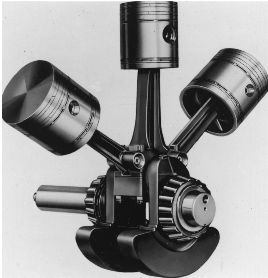
FIGURE 3.44 (b) Commercial application of an articulated connecting rod. The centerlines of the cylinder compressor are arranged radially in a single plane perpendicular to the crankshaft axis for better balance. (Source: Worthington Group, McGraw-Edison Company.)
