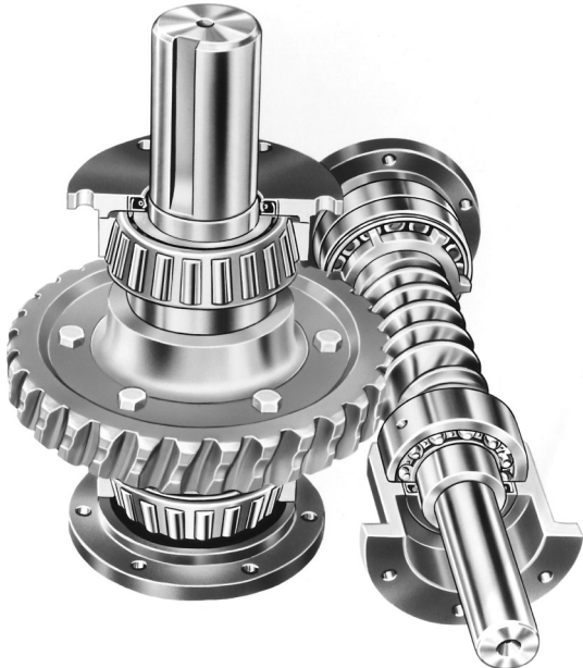
FIGURE 6.6 A worm and worm gear set. The worm gear is a special helical gear used for large reductions in speed. (Source: Cleveland Gear Company.)
