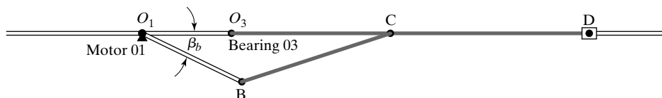
FIGURE 1.24 Quick-return mechanism based on drag link, sample problem 1.7. (a) Limiting position with slider to extreme right.
