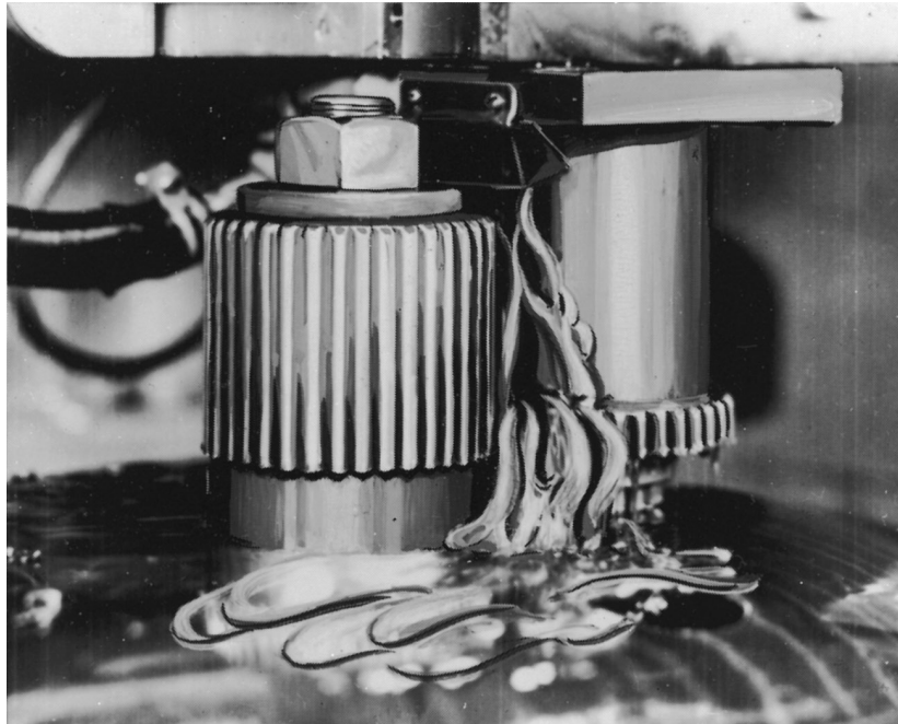
FIGURE 6.23 Generation of a spur gear with a pinion cutter. (Source: Fellows Gear Shaper Company.)
