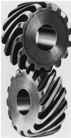
FIGURE 7.8 A pair of crossed helical gears, used when the shafts are not parallel. Usually, crossed helical gears have the same handedness. (Source: Richmond Gear, Wallace Murray Corporation.)
