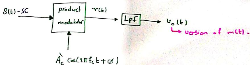
$$\begin{aligned} v(t) &= S(t) A_c \cos(2\pi f_c t + \phi) \\ &= A_c \cos(2\pi f_c t + \phi) \cdot [A_c m(t) \cdot \cos 2\pi f_c t] \\ &= \frac{A_c \cdot A_c}{2} m(t) \cos(4\pi f_c t + \phi) + \frac{A_c \cdot A_c}{2} m(t) \cos \phi \end{aligned}$$
