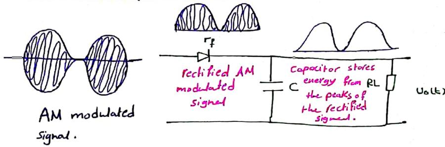
[ Key Ideas: capacitor captures the voltage peaks of rectified wave form ]
