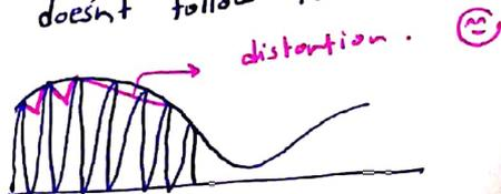
\* Switching Amplitude Modulator.
