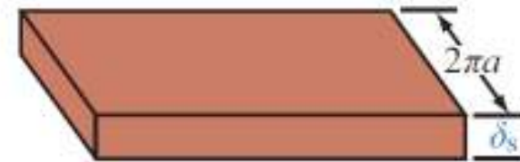
(b) Equivalent inner conductor
