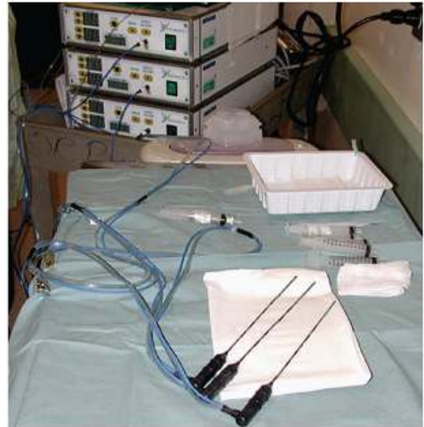
Figure TF4-2: Photograph of the setup for a percutaneous microwave ablation procedure in which three single microwave applicators are connected to three microwave generators. (Courtesy of RadioGraphics , October 2005 pp. 569–583.)
