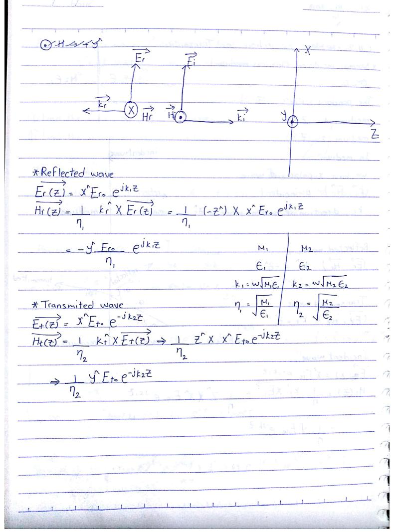
Relating Er. and Eto to Eio All wave have E H fields tanyontional to the boundary. Boundary condition :-Tangential Eard A Fields are continous accross the boundary. Medium - 1  $\overline{E_{i}(z)} = \overline{E_{i}(z)} + \overline{E_{i}(z)} = x^{r} \left( \overline{E_{io}} e^{jk_{i}z} + \overline{E_{io}} e^{jk_{i}z} \right)$ H,(Z) = y (Eio e-jtiz - Ero ejkiz) F2(2) = x E+0 e-jk22 H2(2) = y Eto e-jk22 \* Bondary Condition X (Eis Fro)
