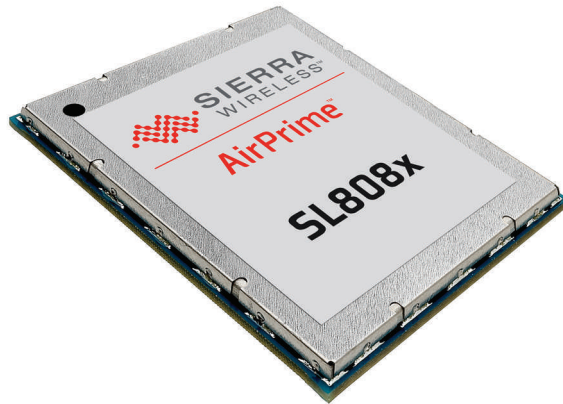
Figure 21-21 The Sierra Wireless AirPrime SL808x embedded cellular module offers 3G HSDPA/GSM/GPRS/EDGE connectivity and quad-band 850/1900/1800/900-MHz coverage. The dimensions are 25 × 30 × 2.35 mm.
