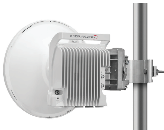
Figure 20-22 The Ceragon FibeAir IP-20C is typical of the small-cell backhaul units available. This one packages the radio, interfaces, and dish antenna into a single unit and is available in standard licensed band frequencies from 6 to 42 GHz. Typical data rate is 1 Gbps in a single Ethernet channel. It uses 2048 QAM.
