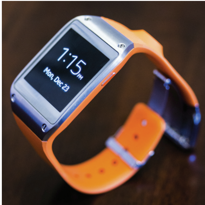
Figure 20-16 The Samsung Gear smart watch communicates with a smart phone with Bluetooth wireless technology.
