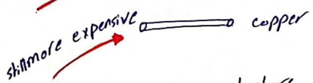
\* we use Aluminum conductors with large cross section area to overcome its higher resistivity.
