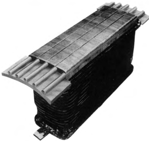
FIGURE 5–17 A rotor field pole for a synchronous machine showing amortisseur windings in the pole face. (Courtesy of General Electric Company.)
