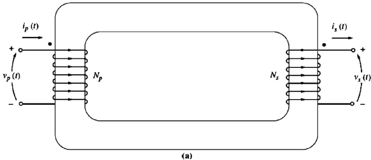
(a) FIGURE 2-4 (a) Sketch of an ideal transformer.
