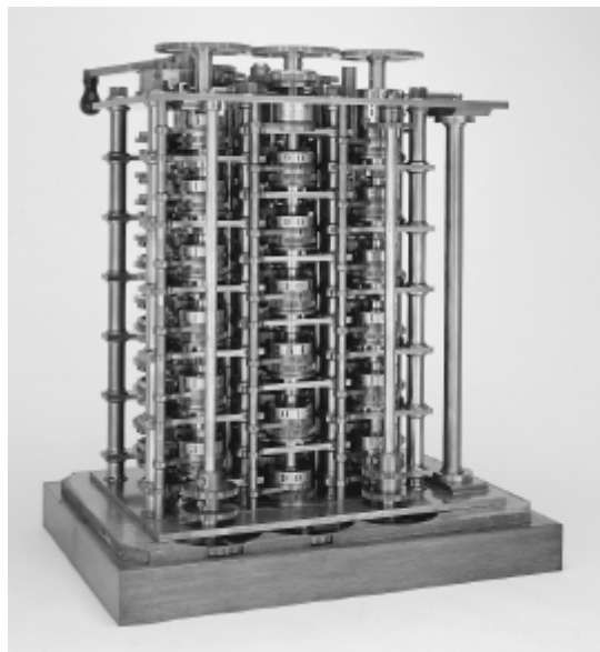
Figure 1.1 Working part of Babbage's Difference Engine I (1832), the first known automatic calculator (from [Swade93], courtesy of the Science Museum of London).
