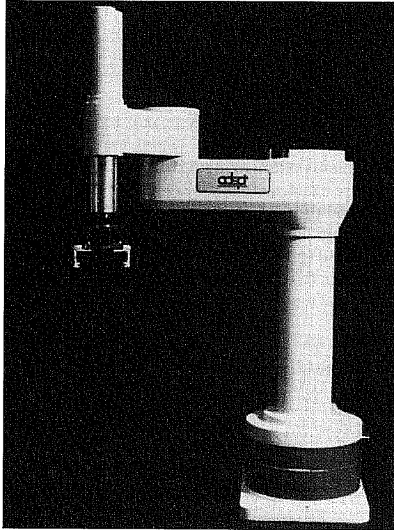
FIGURE 10.9: The Adept One, a direct-drive robot by Adept Technology, Inc.
